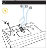
Connect water supply hose to the shower head and connect the power
